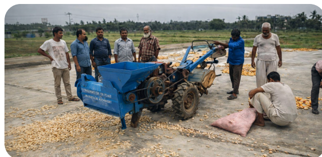
Figure 8. Walkman tractor driven maize sheller
