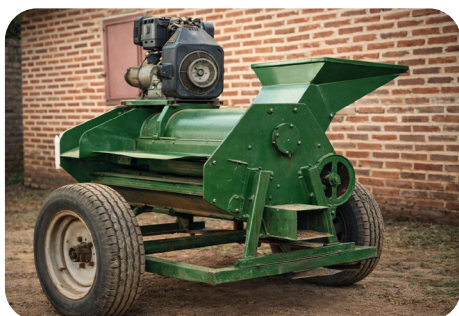
Figure 7. Engine-driven maize sheller (engine mounted on the machine)
