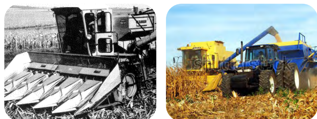
Figure 2. six row corn head and Combine-harvester in operation.
