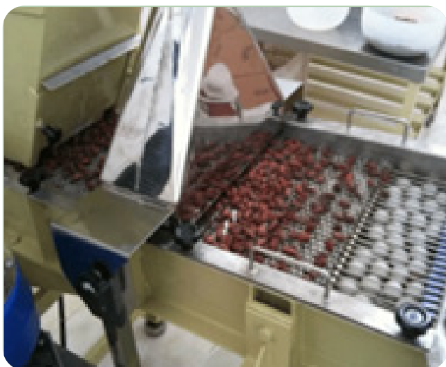
Figure 9: Mechanical bean cleaner
