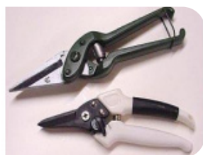
Figure 7. Hoof trimmers for removing obstructs between hooves and removing abnormally growing hooves
